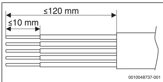
Fig. 24 Wire stripping mains feed connection
