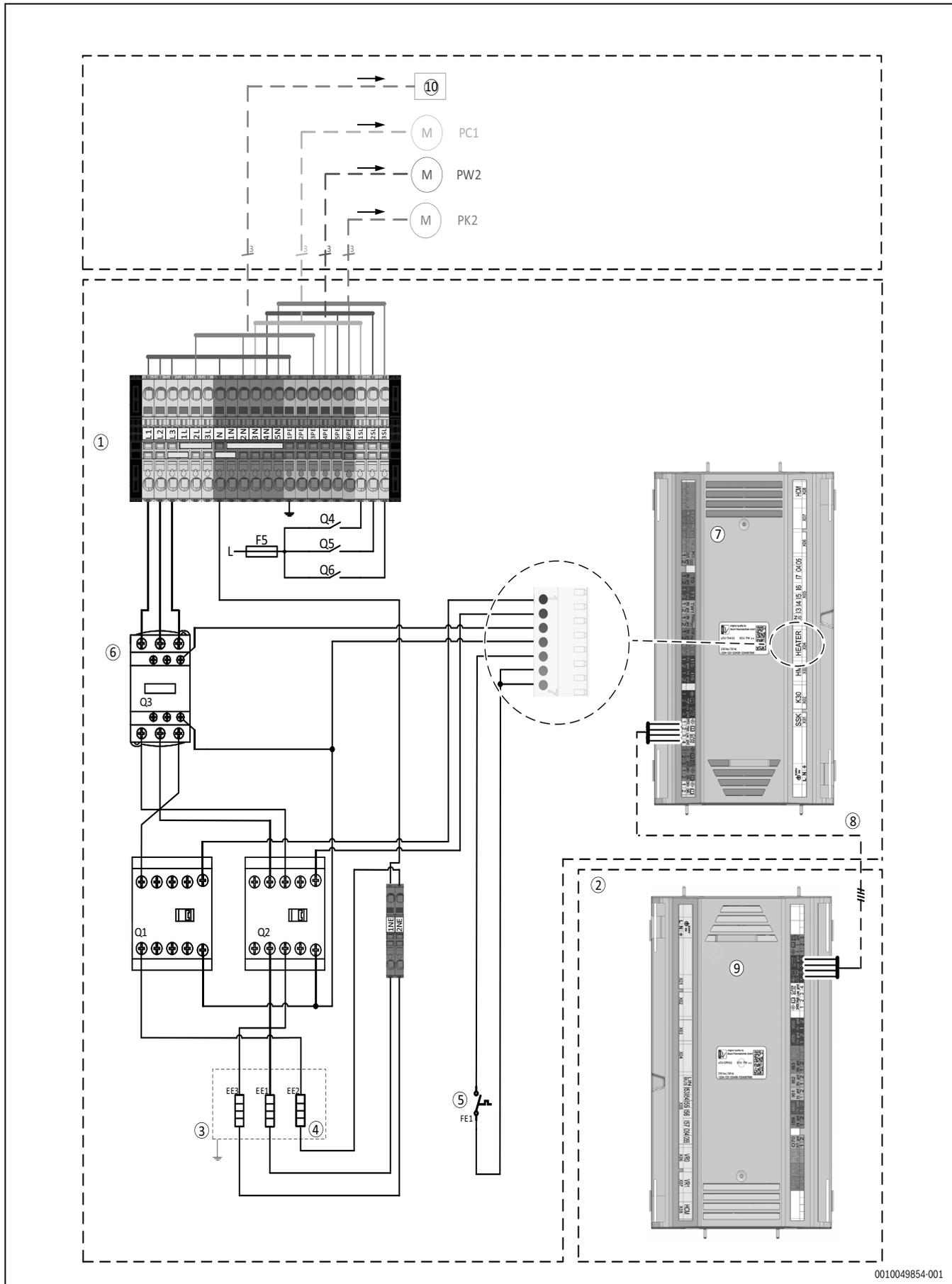
Fig. 41 Power supply indoor unit, standard
