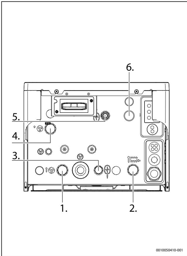
Fig. 14 Pipe connections
