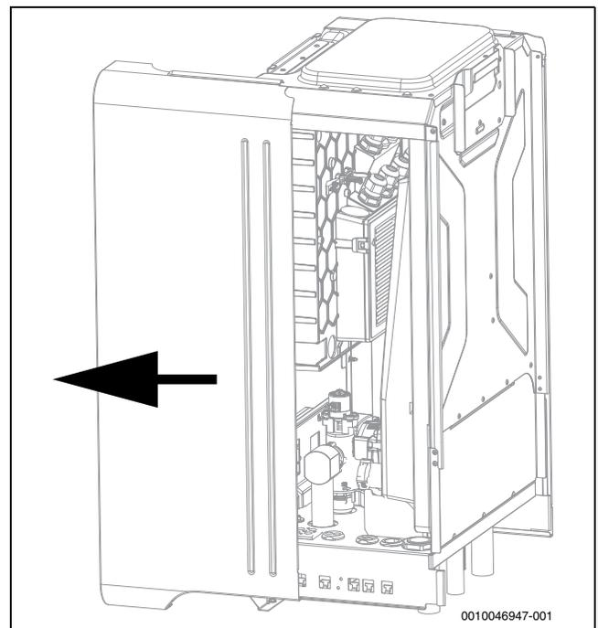
Fig. 13 Remove the side cover
