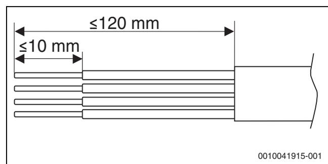
Fig. 21 Wire stripping CAN-BUS
