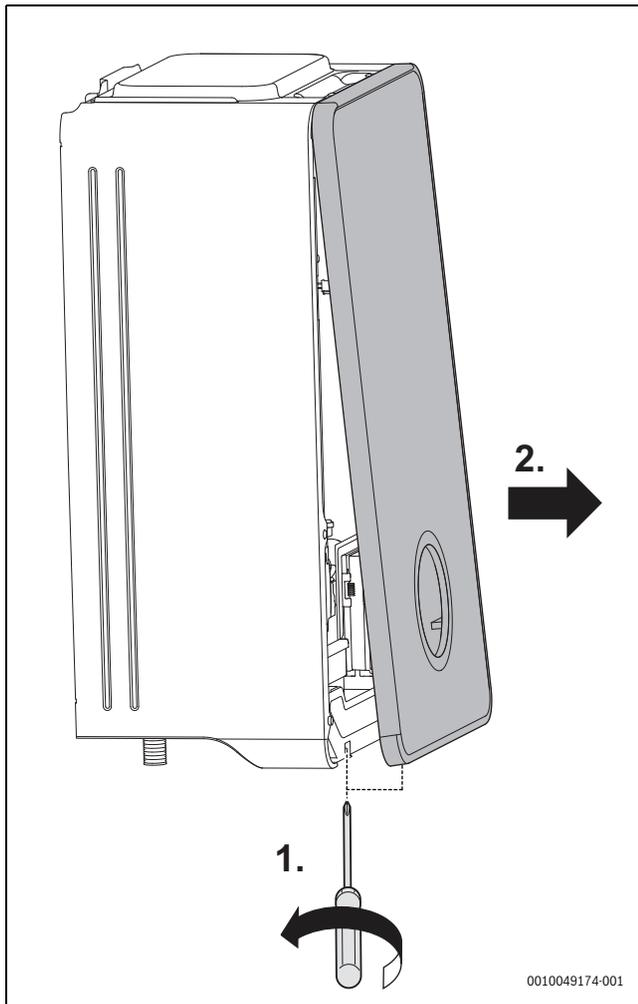
Fig. 10 Remove the front
