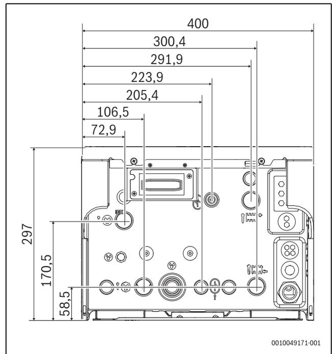
Fig. 3 Dimensions connections, bottom view (mm)
