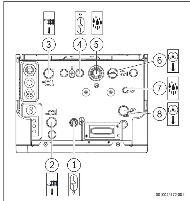
Fig. 6 Pipework connections
