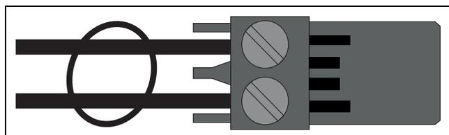
Fig. 34 Cable tie on connector
