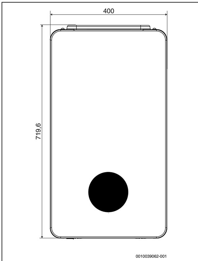
Fig. 2 Dimensions front view (mm)
