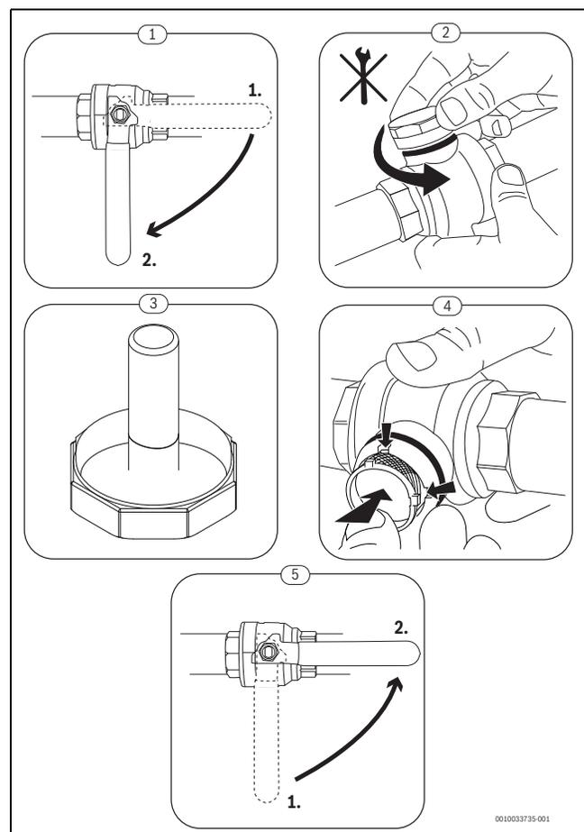
Fig. 36 Cleaning the strainer
