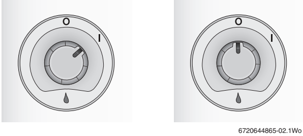
Fig. 3 Switch off central heating
